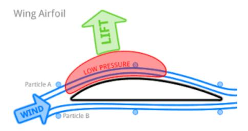
The above diagram shows how the wing of an airplane works. Sails essentially work the same way, creating lift which will cause the vessel to move forward.
